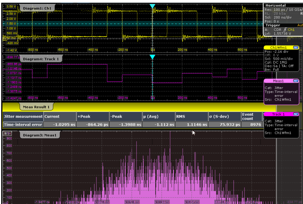
Figure 15-1: TIE measurement with CDR trigger, 10 Mbps, with track and histogram
